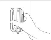
6. Determine mounting location for the light. Place the mounting plate on the surface so that the tab is pointing down and mark the pilot holes for drywall. Use a drill to insert the anchors, then line up the mounting plate with the holes and drill screws in.
