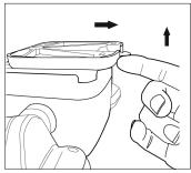
1. To remove the back plate from the light, use your finger to push up on the mounting bracket tab. This will unlock the bracket. Then slide the bracket down off the back of the light.
