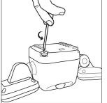
2. Use a screwdriver to loosen the four screws on the back plate. The screws will not come out all the way.
