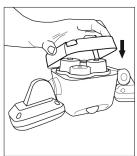
4. Replace the battery lid and make sure the screws are twisted in tightly.
