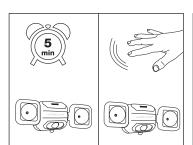
5. Before mounting your light, test the motion sensor in a dark closet or bathroom. Close the light in the dark room and leave for up to 5 minutes. When you re-enter the room, the light should activate with motion
