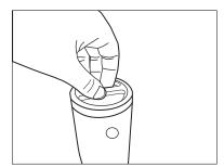
2. Twist the lid counterclockwise to unlock.
