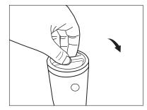
5. Once the batteries have been inserted, replace the lid by lining up the arrows and turning until the arrow is pointing towards the lock symbol.
