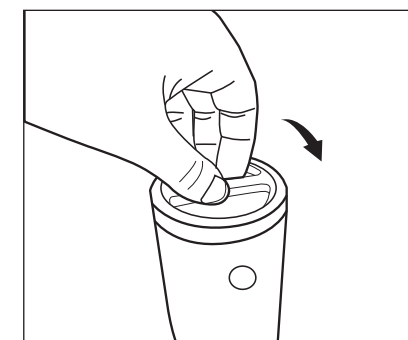
5. Once the batteries have been inserted, replace the lid by lining up the arrows and turning until the arrow is pointing towards the lock symbol.
