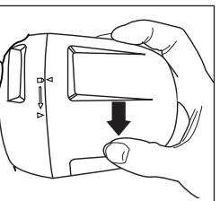
1. Remove the face of the light by rotating counter-clockwise as shown above.
