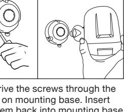
10. Drive the screws through the holes on mounting base. Insert the stem back into mounting base and tighten the thumbscrew.
