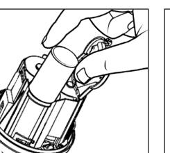
4. Insert 3 D-cell batteries with correctly polarity. Make sure the flat ends of the batteries are against the springs.
