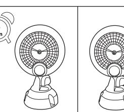
7. Test the motion sensor in a dark closet or bathroom. Leave the light in the dark room for up to 5 minutes. When you re-enter the room, the light should activate with motion.
